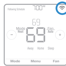
Example of thermostat included and connected in a Z-Wave network.
